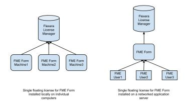
If the expiry dates associated with multiple FME installation serial numbers vary, the floating license applies the shortest expiry date to all serial numbers.
