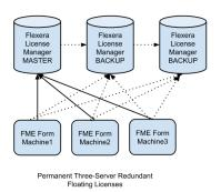
It is not a requirement for each of the server nodes to have the same architecture or operating system, although they should have reliable network communications with each other and should be on the same subnet. Often, this means that the three servers are located physically close to each other.
