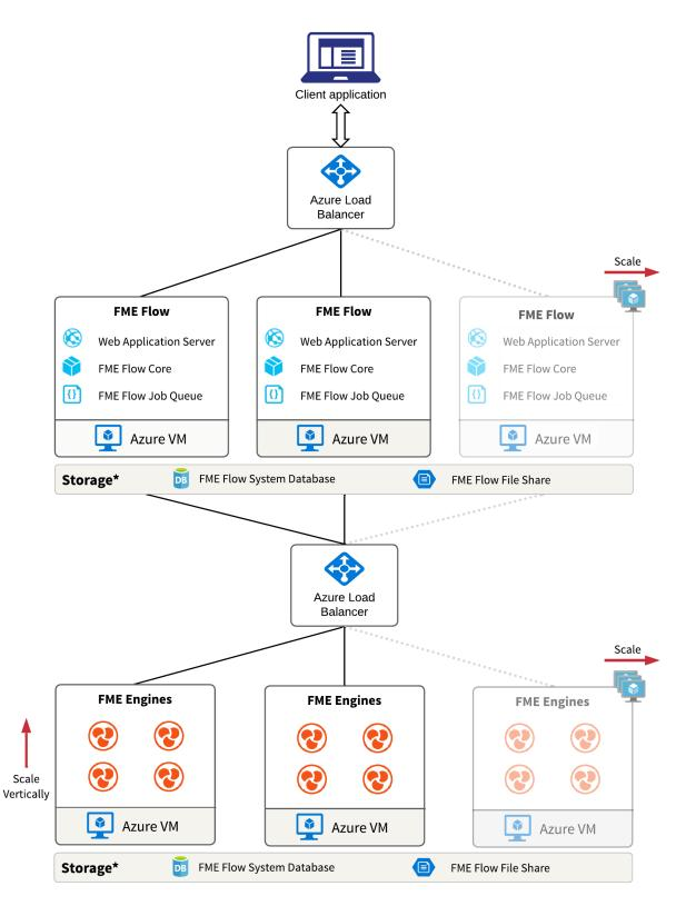
\* The same FME Flow database and file share need to be accessed by both the FME Engine VM and the FME Flow Core VM.
