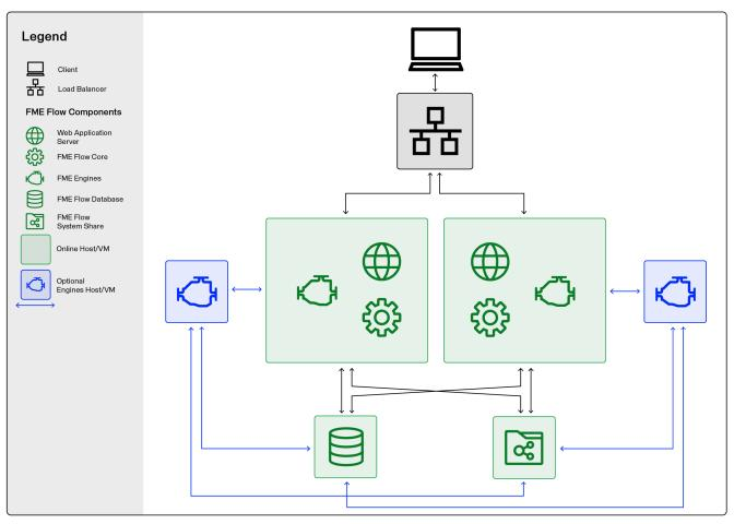
Fault Tolerant Install Example 3
