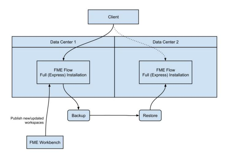
Keep in mind that when planning for disaster recovery, all clients of FME Flow, including web browsers, the <u>FME Flow CLI</u>, and the <u>FME Flow REST API</u>, must connect to the "active" FME Flow Core host.
