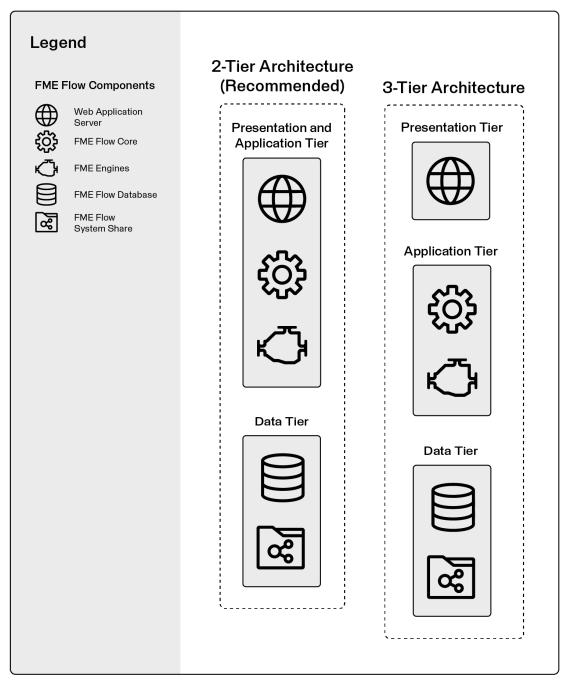
In a 2-tier architecture, an Apache Tomcat web application server runs the <u>FME Flow Web</u> <u>Services</u>, and is installed alongside the the <u>FME Flow Core</u> and <u>FME Engines</u>. Only the <u>FME Flow Database</u> is installed separately, along with a remote file system for the FME Flow System Share.
